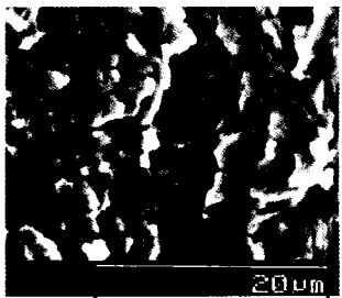
Photo 5 Striation of fatigue crack propagation by SEM (Un-peening, RT)
