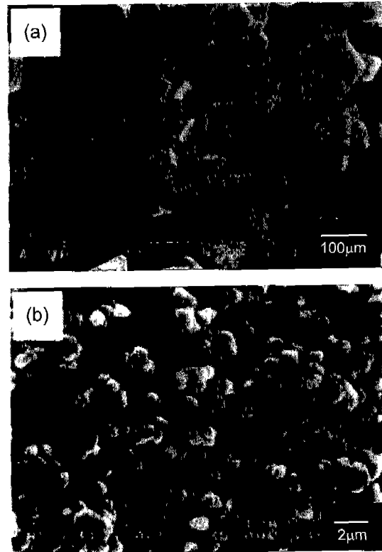
Fig. 1. SEM morphologies of (a) WO_3 and (b) CuO powders.
