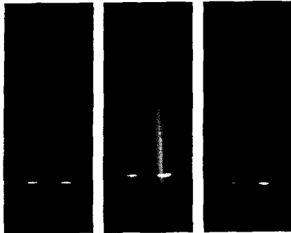
Fig. 3 Unstable flames in a oxidizer deficient ambience ( Q_{fuel}=94.5 cc/min, Q_{air}/Q_{sto.}= 0.80 )
