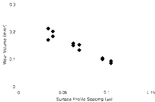
Fig. 5 Effect of surface profile spacing on the wear volume
