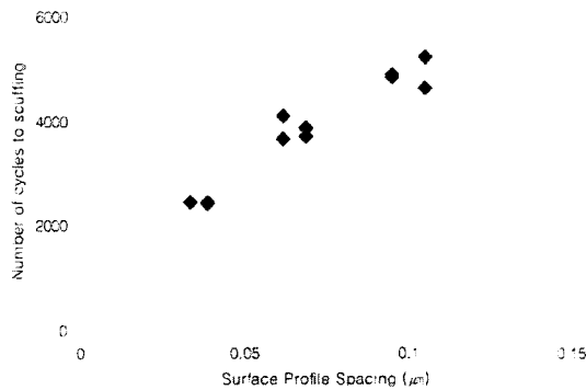
Fig. 4 Effect of surface profile spacing on the number of cycles to scuffing
