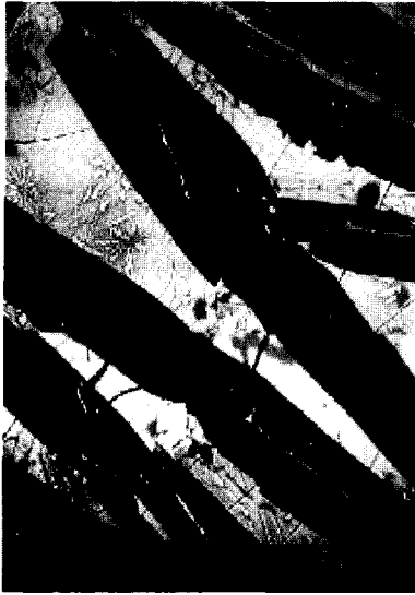
Fig. 8. SEM micrograph of Curragh slag after viscosity measurements.
