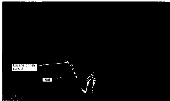
Fig. 7. Escaping behaviour of fish school below the lead line obtained by the scanning sonar.
