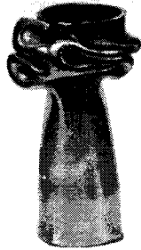
(a) Tube type energy absorber
