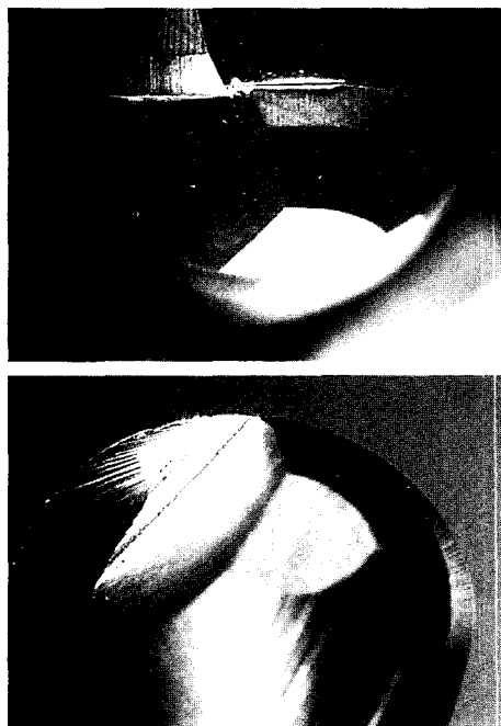
Fig. 6. Wear types at the tool edge.
