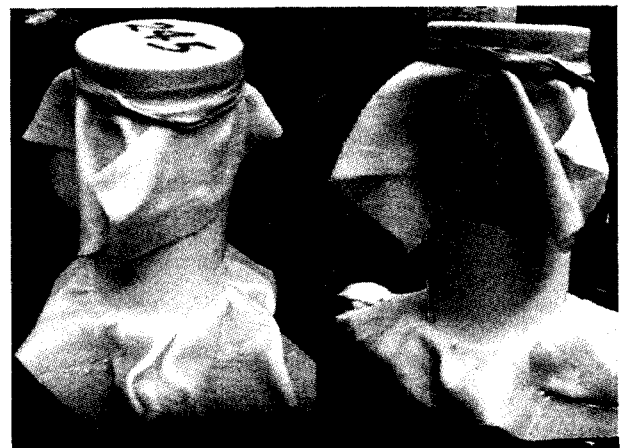
Fig. 6. Samples with fabric on ends for water curing
