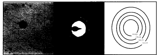
Fig. 6 STEM micrograph and electron diffraction ring patterns of BN precipitate in simulated HAZ of Steel C
