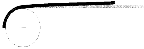
Fig. 16(b) Post-forming deformation with stress relieving. Tensile force was not applied
