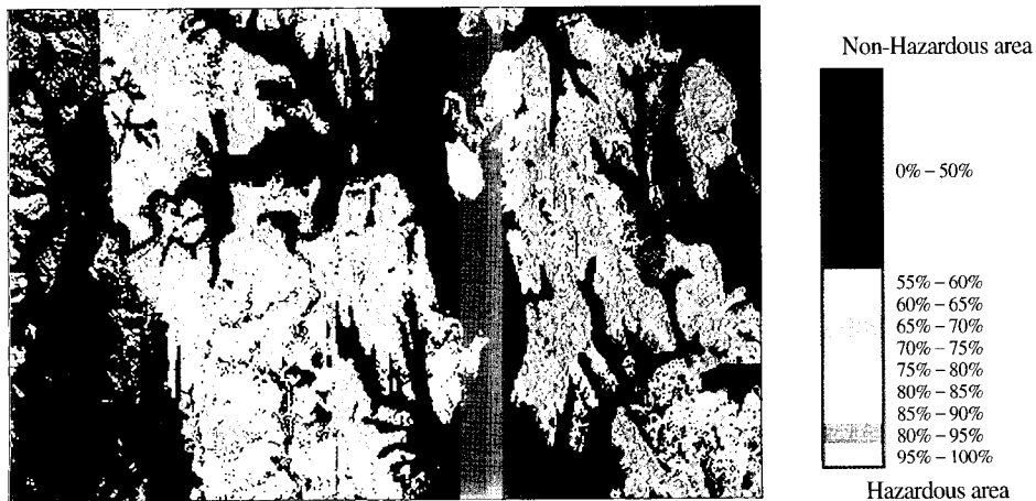
Fig. 5. Prediction map of landslide hazard in Boeun area using the likelihood ratio function.
