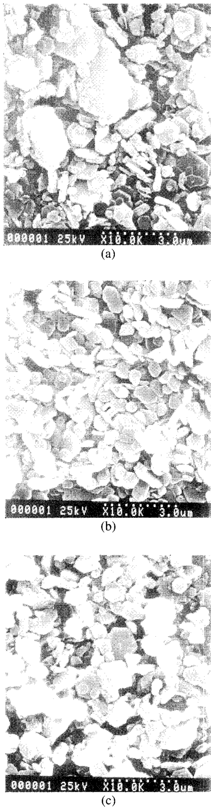
Fig. 2. Scanning electron micrographs of various MDH: (a) unmodified, (b) aliphatic long chain-modified, and (c) amino silane-modified.
