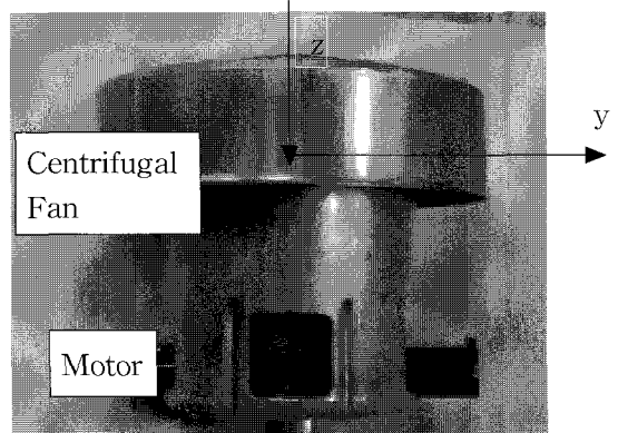
Fig. 2 Overview of the centrifugal fan used in a vacuum cleaner
