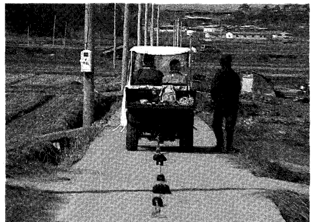
Fig. 4. A picture showing continuous data measurement with CCR system.
