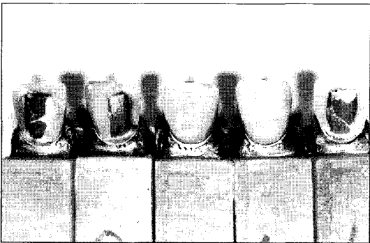
Fig. 6. Fracture pattern of Artglass crowns.
