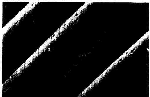
(c) 25% NaOH treatment (60°C, 60min.) - 22% weight loss
