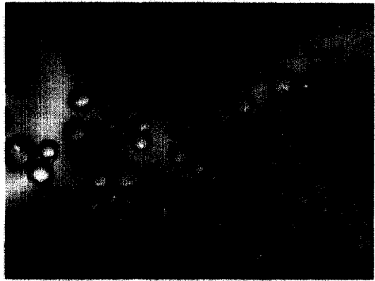
Fig. 7. Microphotograph of microcapsule with tetradecane(8000 rpm).
