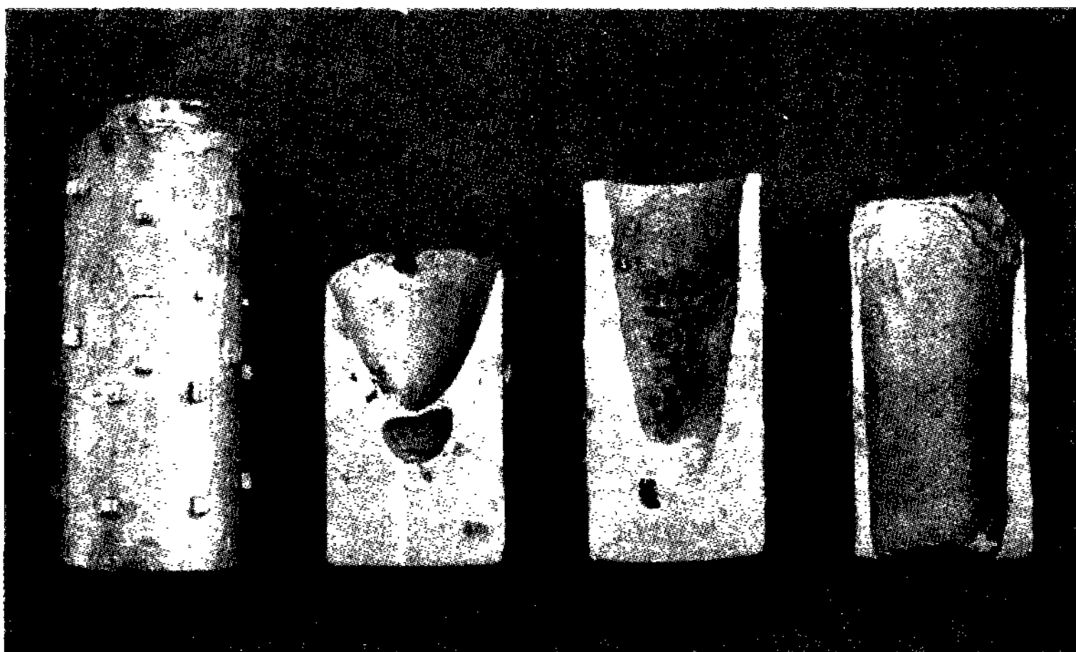
Fig. 4. The effect of revolution speed on the solidification profile of runner. *overflown for 800 rpm
