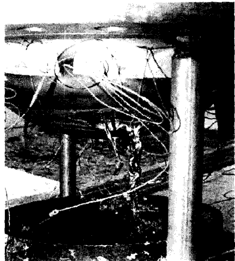
Fig. 8 Vessel failure by the thermal attack of the alumina and iron melt.
