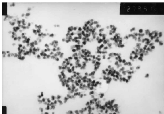
Figure 1. Transmission electron micrograph, showing Fe nanoparticles of 80-110 \text{\AA} in diameter in a cellulose acetate film
