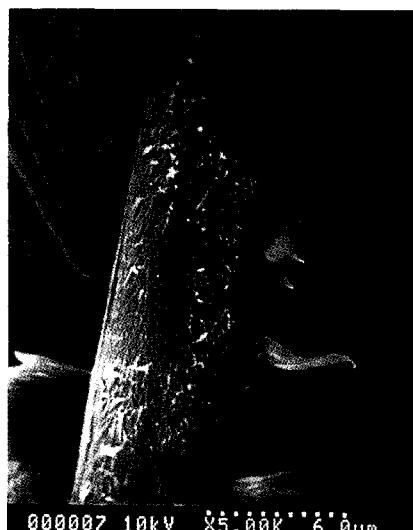
**Figure 8.** Fracture surfaces of (a) CF(S)/HDPE and (b) CF(U)/HDPE.
