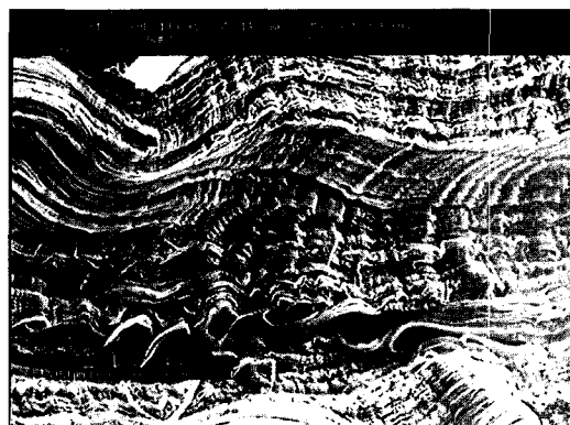
Figure 5. Scanning electron micrograph of the fractured surface of LLDPE.
