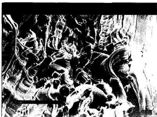
Figure 6. Scanning electron micrograph of the fractured surface of the rice starch-LLDPE composite.
