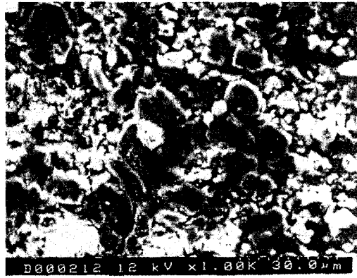
a) Micrograph of surface corrosion
