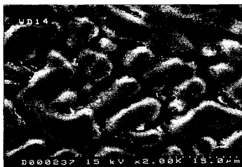
c) SEM micrograph of interdendritic corrosion on the surface
