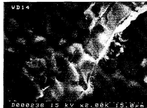
b) SEM micrograph of corrosion between droplets
