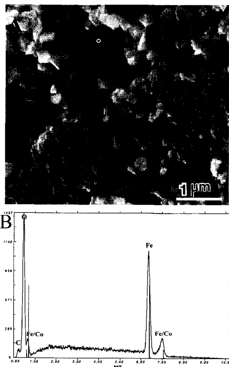
Fig. 4. Scanning electron micrograph (a) and the energy dispersive X-ray analyses (b) of Ni-incorporated magnetite. Residual salt from microbial media coexisted with magnetite crystals.
