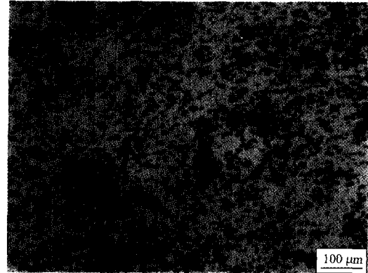
Fig. 2. Optical microstructure of Al/SiC composite for a constant particle size.
