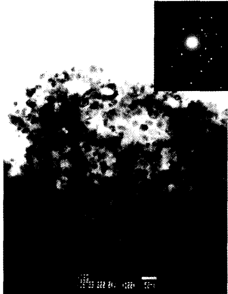
Fig. 4. TEM photograph and SAD pattern of the Ni particles.
