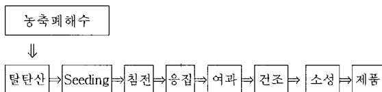
Fig. 1. Schematic diagram in recovering of magnesium from waste bittern.
