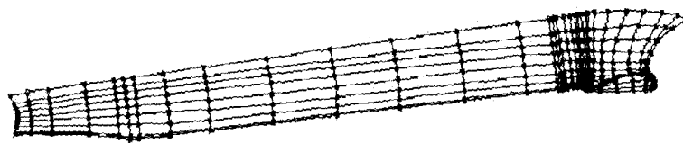
Figure 2: The B-spline surface control net of the model of Figure 1
