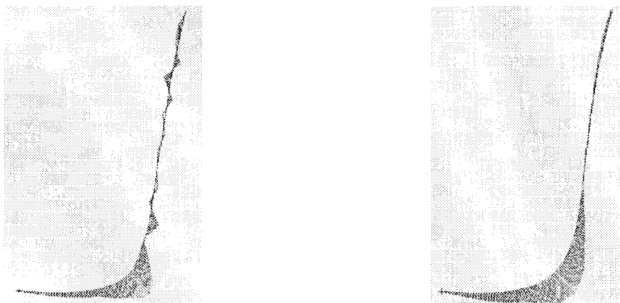
Figure 6: Porcupine plots of the initial(left) and the faired(right) Station 2, created in Autoship
