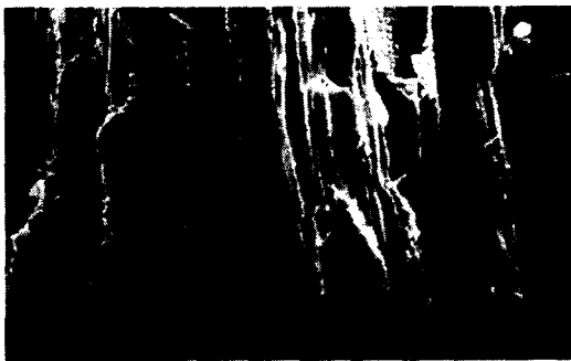
Fig. 10. Scanning electron micrograph(SEM) of NaOH treated wood mill of Suwon poplar after enzymatic hydrolysis.
