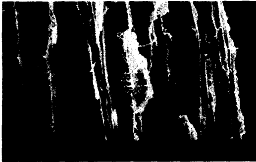
Fig. 9. Scanning electron micrograph(SEM) of untreated wood mill of Suwon poplar after enzymatic hydrolysis.
