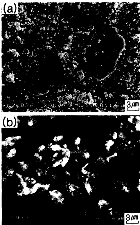
Fig. 3. SEM morphologies of (a)W-CuCl 2 , and (b)WO 3 -CuCl 2 powders prepared by the slurry mixing and the ball milling and slurry mixing respectively.
