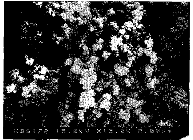
Fig. 2. Particle size distribution and SEM micrograph of as-received zirconia powder.
