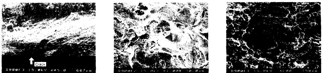
(a) Crack initiation (b) Striation and brittle fracture (c) Dimple Fig. 13 SEM fractography on the fracture surface (degraded 220MPa)
