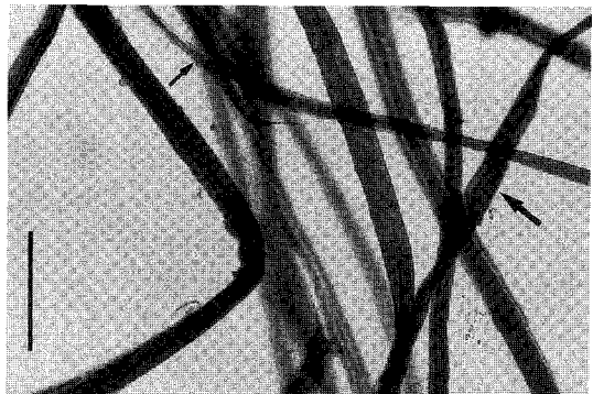
Fig. 4. Transparent membrane separated from paper mulberry fibers in sample 3. The bar represents 100 micrometers.
