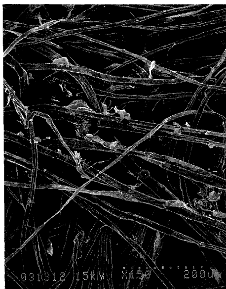
Fig. 9. Condition of paper mulberry fibers in paper structures (sample 3). Transparent membrane on the fiber surface (arrows).
