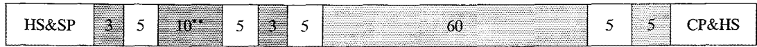
Figure 1b. Configuration of 0.25 ml straw loaded before vitrification. unit (mm); [HS&SP]: heat sealing & sealing powder, [25% glycerol + 25% ethylene glycol]: 25% glycerol + 25% ethylene glycol, [10**]: embryo column, [ ]: air, [0.5 M sucrose]: 0.5 M sucrose, [CP&HS]: cotton plug & heat sealing.
