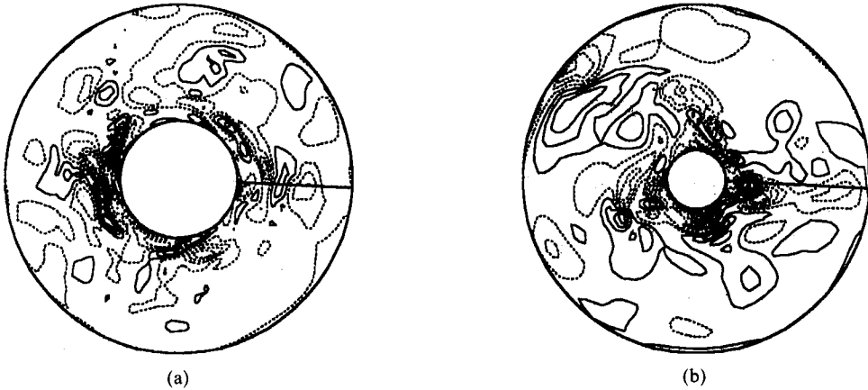
Fig. 6 Contours of normalized streamwise vorticity ( \omega_3 v/u_r^2 ) on a plane normal to the mean velocity at z=2\pi . (a) \delta/a=2 (b) \delta/a=5
