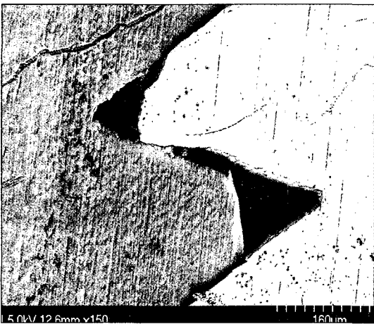
Fig. 8. Crevice corrosion behavior of sample using screw after CPPT in SEM. (A: abutment, F: fixture, G: gold screw)
