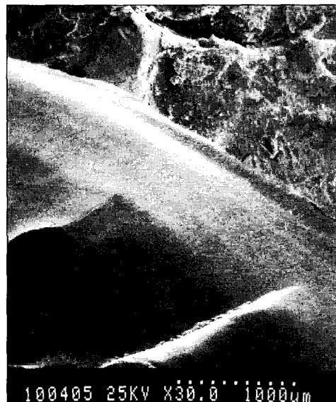
Fig. 4. SEM photographs showing fracture surface of Targis group.
