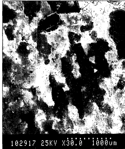
Fig. 6. SEM photographs showing fracture surface of Sculpture group.
