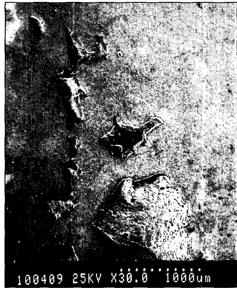
Fig. 5. SEM photographs showing fracture surface of Artglass group.
