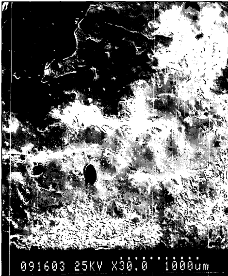
Fig. 6. SEM photographs showing fracture surface of Sculpture group.
