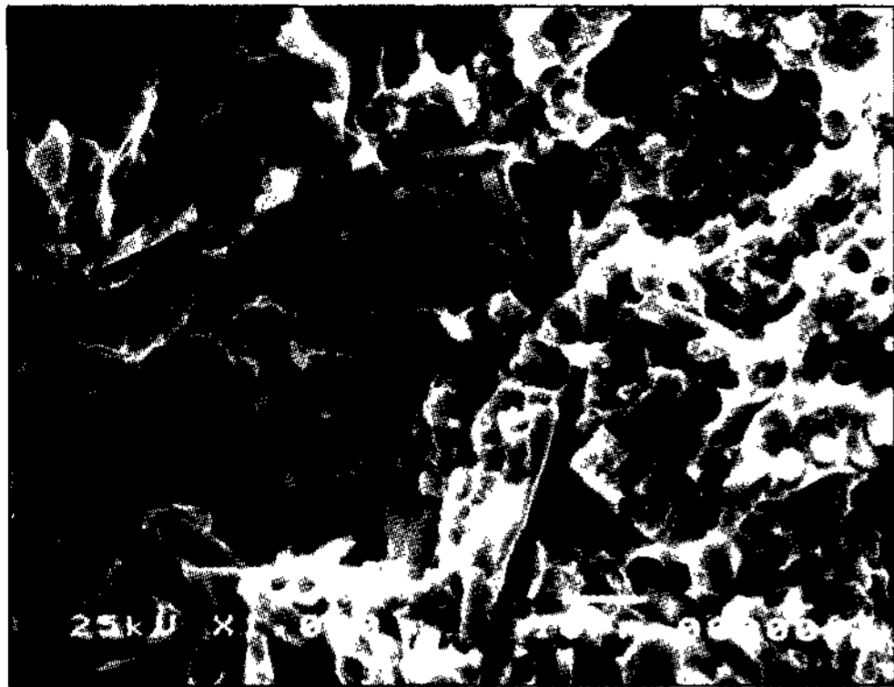
Fig. 12. SEM fractograph of the tensile test specimen of (Al 2 O 3 + Si)/AZ91 matrix composites.
