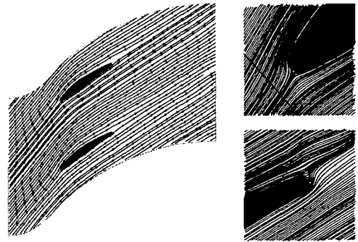
Fig. 7 Computed streamline inside blade passages
