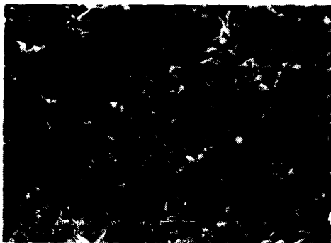
Fig. 18. Machined surface with 4~8 \mu\text{m} slurry
