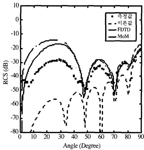
Fig. 3. RCS of a  $3\lambda$ -long conducting cylinder
