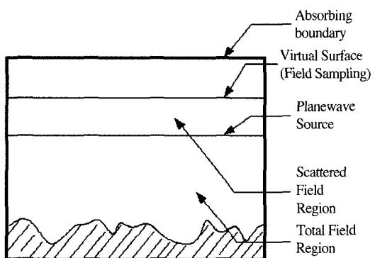
Fig. 5. FDTD analysis region for a distributed target.
