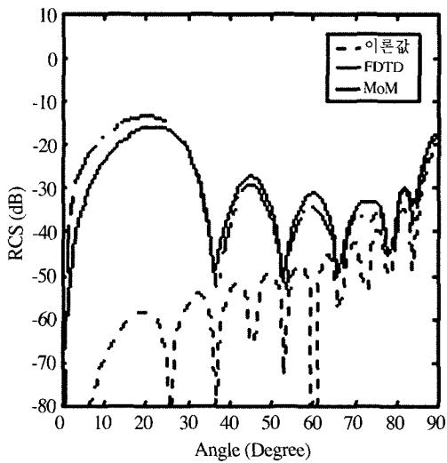
Fig. 4. RCS of a  $5\lambda$ -long conducting cylinder
