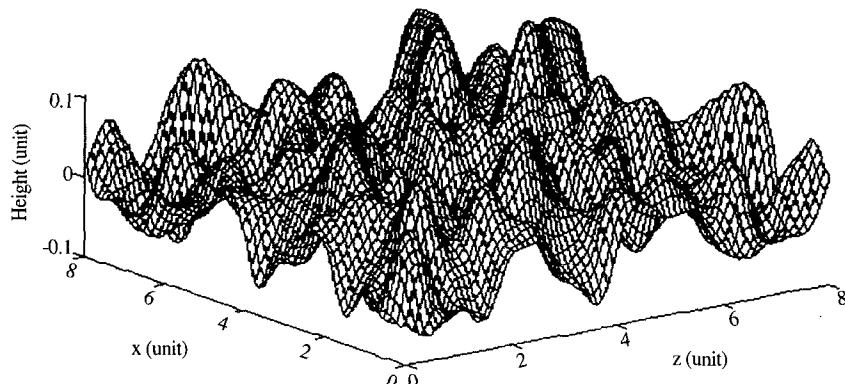
Fig. 7. A typical profile of a randomly rough surface.
