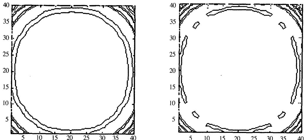
Fig. 6. Comparison of the absorbing boundary conditions; (a) PML ABC and (b) Mur's 2nd ABC.
