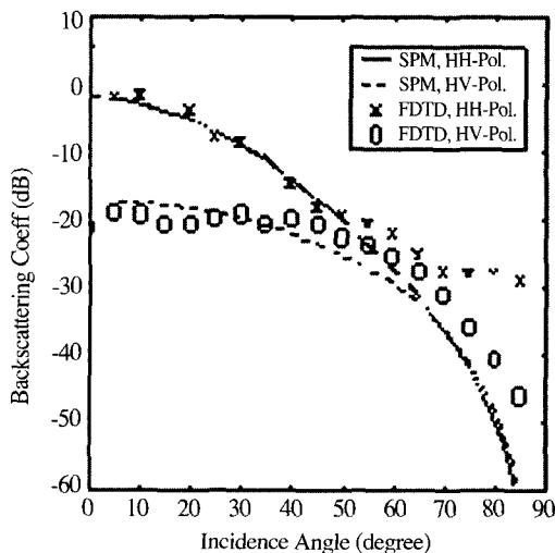
Fig. 8. Backscattering Coefficient of a conducting rough surface.
