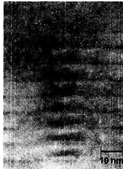
Fig. 2. High resolution STEM image of multilayered InAs quantum dots.
