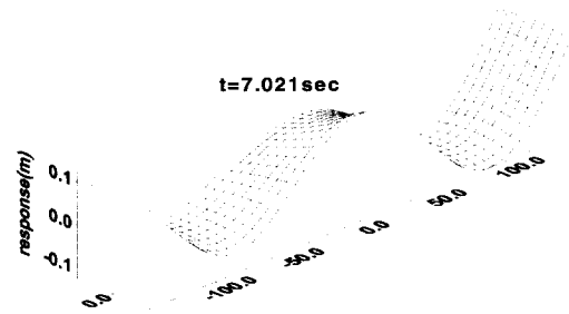
Fig. 8 Distribution of vertical displacement amplitude by aircraft collision
