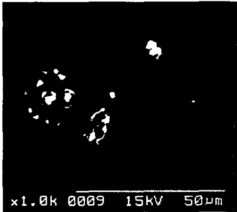
Photo. 1. Pitting at 316L stainless, after cyclic polarization in 3.5% NaCl solution.(x 1,000)
