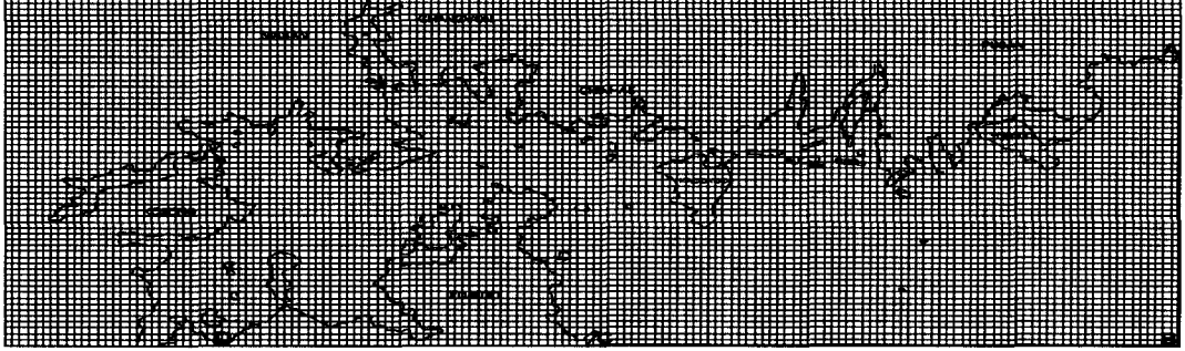
Fig. 2. The finite-difference grid of the three-dimensional model in the study area.
