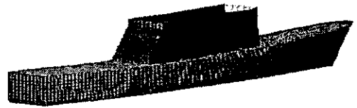
Fig.9 Patch distribution of ship before shaping
