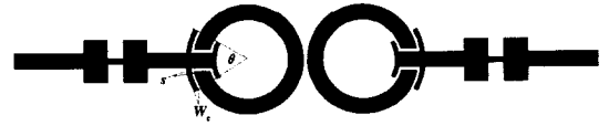
Fig. 1. The new microstrip two-stage two lines-to-ring bandpass filter with lowpass filter at feedlines.
