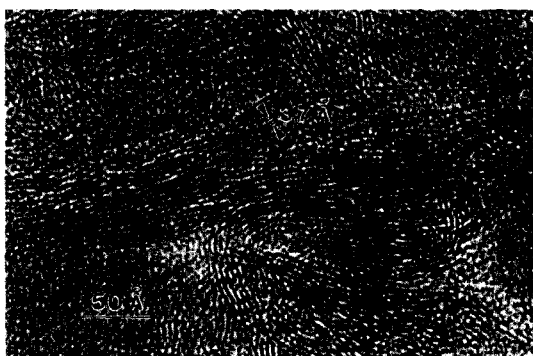
Fig. 5. HRTEM image of discrete carbonaceous material showing a "fingerprint" texture. Carbonaceous layers are wavy and circular in part.
