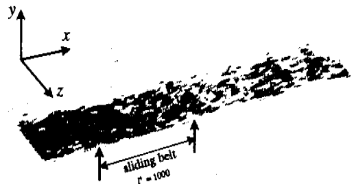
Fig. 8 Iso-surfaces of instantaneous streamwise vorticity. \omega_x v / u_\infty^2 = -0.25 (black) and 0.25 (grey).
